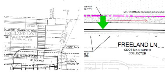
3. Revise the site plan and conditional note(s) to reverse the direction of the proposed one-way driveway and internal street network to provide the egress movement on Ellenwood Place and the ingress movement on Freeland Lane.
