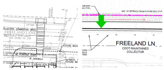
3. Revise the site plan and conditional note(s) to reverse the direction of the proposed one-way driveway and internal street network to provide the egress movement on Ellenwood Place and the ingress movement on Freeland Lane.
