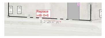
7. Outstanding Comment From 02-24-22: Revise site plan and conditional note(s) to commit to removal of the existing driveway and replacing the curb and gutter per the Chapter 19 Ordinance requirements. Reference Charlotte Land Development Standards Manual detail 10.17A on plan.
