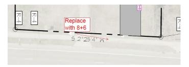
7. Outstanding Comment From 02-24-22: Revise site plan and conditional note(s) to commit to removal of the existing driveway and replacing the curb and gutter per the Chapter 19 Ordinance requirements. Reference Charlotte Land Development Standards Manual detail 10.17A on plan.
