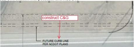
b. **Rigsby Road:** Curb and gutter will be constructed in accordance with CLDSM U-05A, Local Commercial Wide cross section with the back-of-curb located 20.5-feet from the existing centerline.
