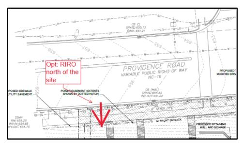
4. Revise site plan and conditional notes to commit to dedicate 50-foot right-of-way from the Providence Road centerline. The site plan shall label and dimension the right-of-way from the road centerline. (refer to Note 6. figure)
