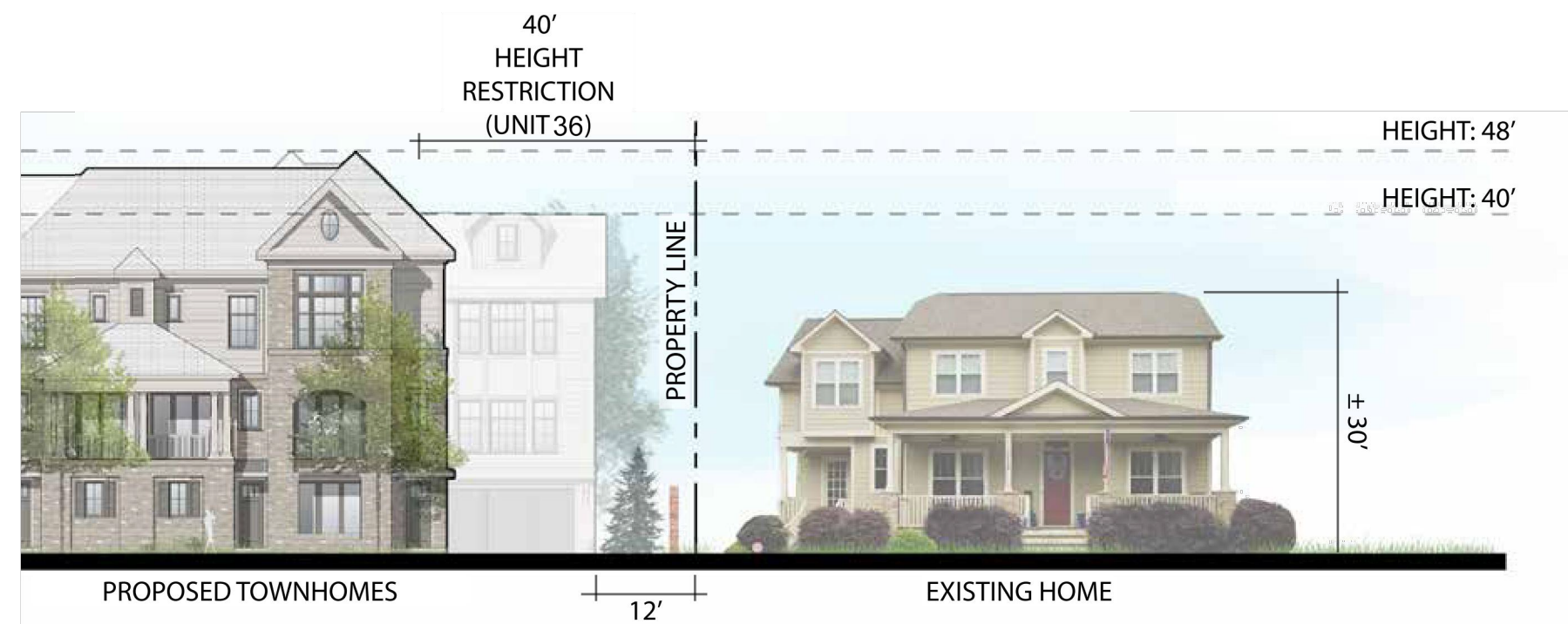
ELEVATION A VIEW FROM PINEHURST PLACE
