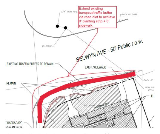
5. The petitioner should revise the site plan and conditional note(s) to commit to constructing an 8-foot sidewalk along the Park Road frontage per Chapter 19<sup>th</sup>. The site plan should label and dimension both items from the back of curb and gutter and road centerline.
