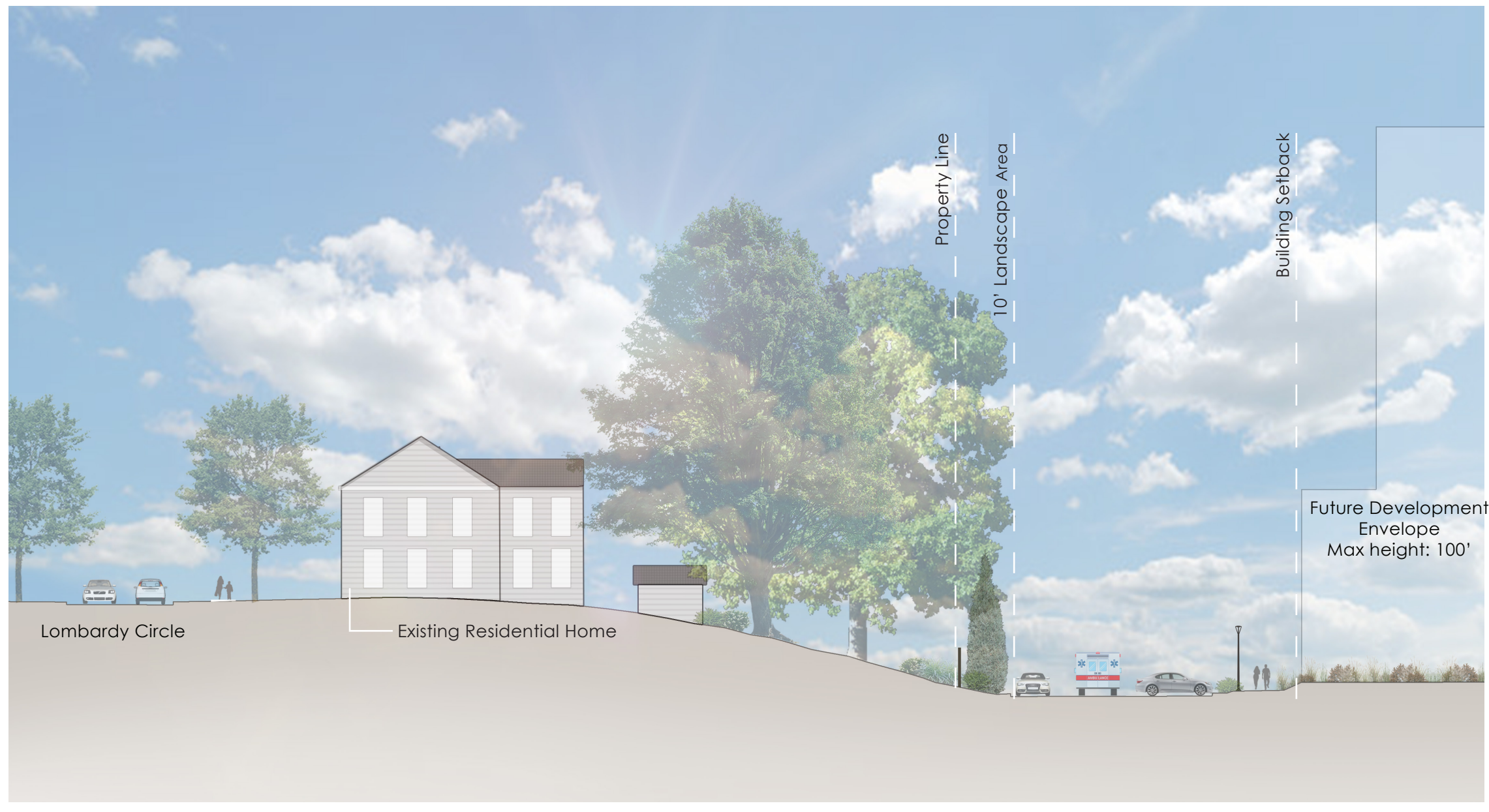
Proposed Landscape Area Section A Atrium Health Main Campus- Charlotte, North Carolina
