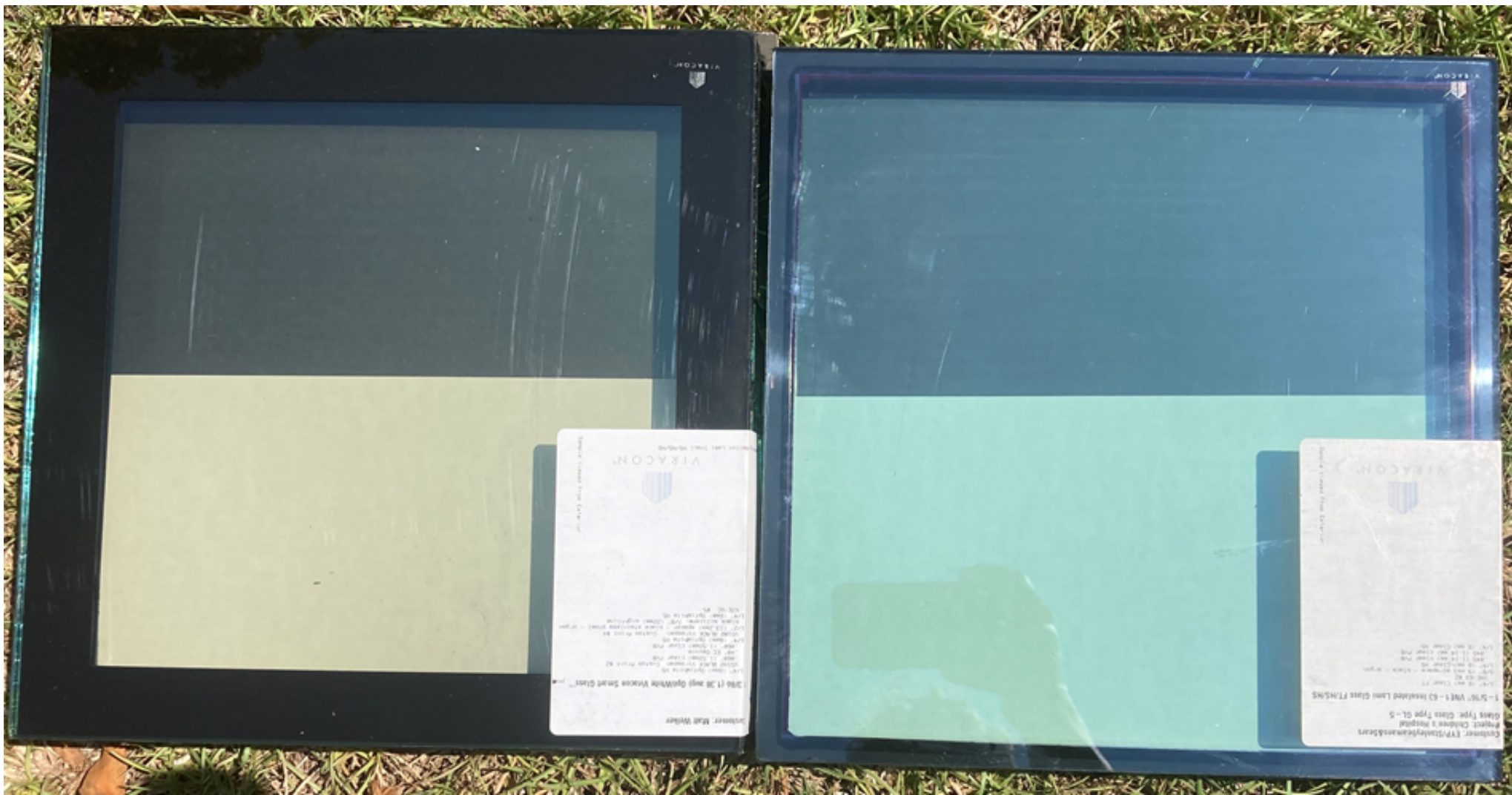
Halio Viracon glass with EC shade device.
