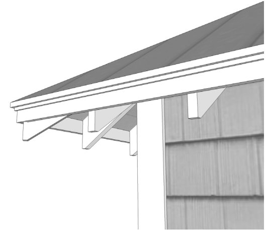
Craftsman style trim details may include corner boards and exposed rafter ends.
