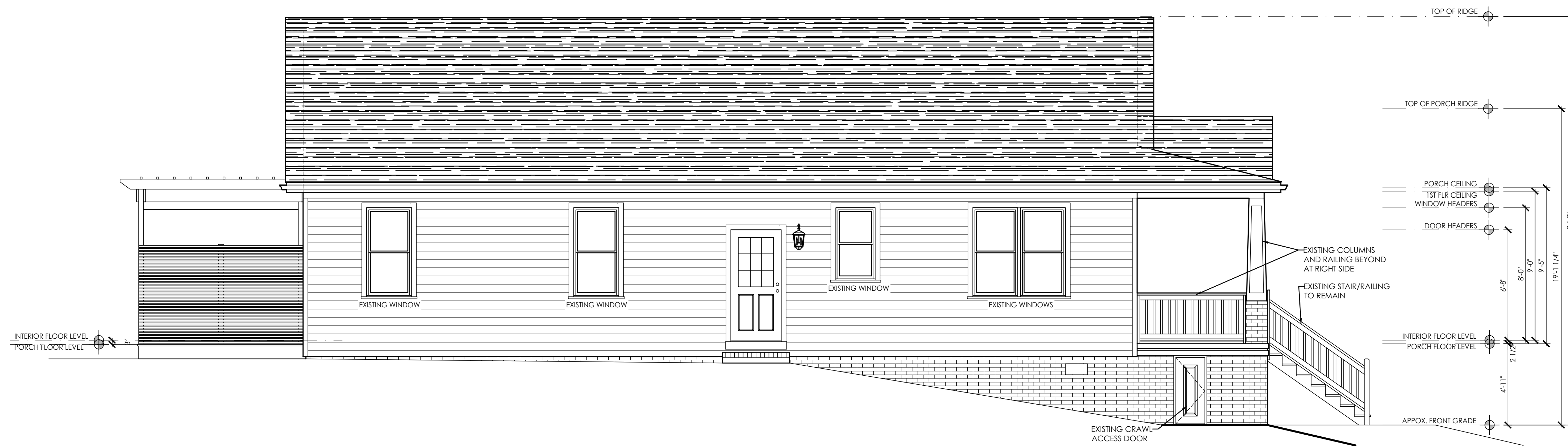
1 EXISTING/AS-BUILT LEFT ELEVATION 1/4" = 1'-0"
