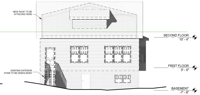
3 EXISTING REAR ELEVATION 1/16" = 1'-0"
