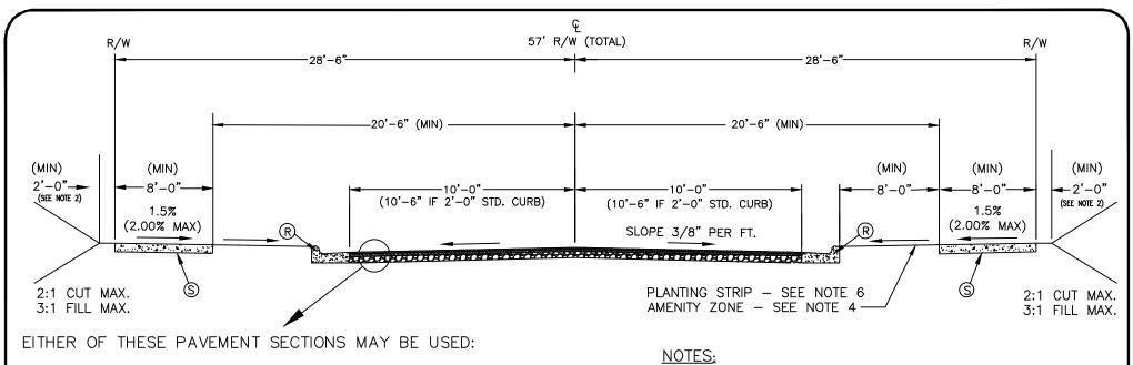
3" BITUMINOUS CONCRETE SURFACE COURSE, TYPE S9.5C TO BE PLACED IN TWO 1.5" LIFTS EACH INTERMEDIATE COURSE 2.5" BITUMINOUS CONCRETE INTERMEDIATE COURSE, TYPE I19.0C 8" COMPACTED AGGREGATE BASE COURSE (USE 6.5" COMPACTED ABC UNDER CURB & GUTTER)
