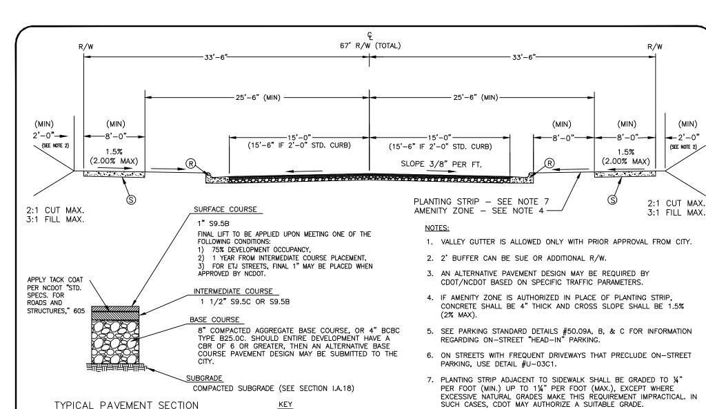
2'-6" STANDARD CURB AND GUTTER, 2'-0" STANDARD CURB AND GUTTER, OR 2'-0" VALLEY GUTTER (SEE NOTE 1)
