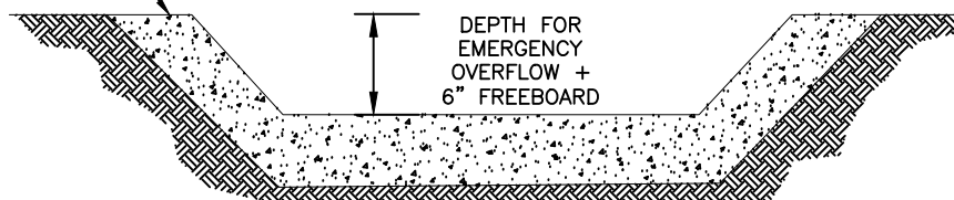
EMERGENCY SPILLWAY DETAIL
