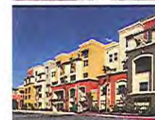
UNDULATION/VARIATION IN FACADE & MATERIAL TO HELP BREAK UP LARGE SCALE OF BLDG
