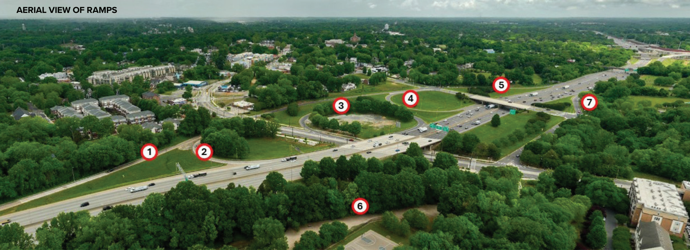
The West End interchange includes seven ramps. For the I-77 southbound direction, several of these ramps are redundant, with five ramps serving two primary movements. (Image: Benjamin Boomers via Google. May 2022.)
