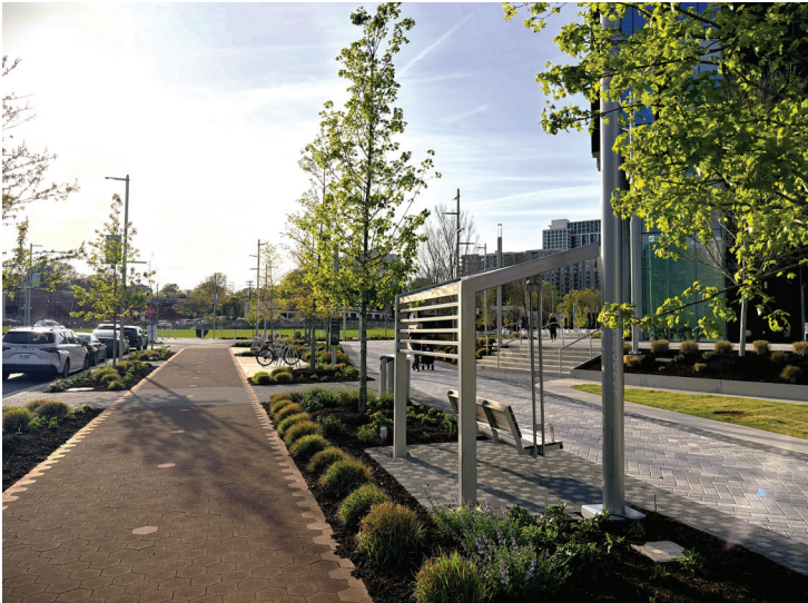
Pearl Park Way was recently completed in the Brooklyn Village / Midtown area of Charlotte. The design of this street, with a wide sidewalks, a raised two-way cycle track, bioswales, and on-street parking is an ideal precedent for the design of the proposed Summit Avenue extension.
