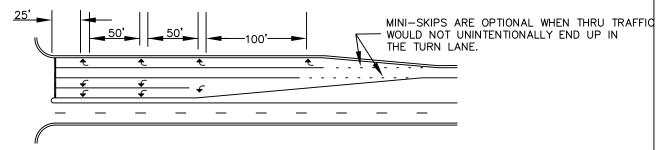
DROP TURN LANES: DROP TURN LANES SHALL HAVE ARROWS AND "ONLY" LEGENDS. THE NUMBER AND LOCATION OF THE ARROWS AND THE "ONLY" LEGENDS SHALL DEPEND ON THE POSTED SPEED LIMIT EXCEPT WHERE THE DROP TURN LANE IS ON THE STEM OF A T — INTERSECTION.
