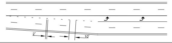
MINI-SKIP LINE THROUGH INTERSECTION: MINI-SKIP LINES SHALL BE SEPARATED BY 6' GAPS WHEN USED THROUGH AN INTERSECTION, i.e. FOR DUAL TURNS OR TO DELINEATE AN OFFSET. ENGINEERING JUDGEMENT SHOULD BE APPLIED WHEN MINI-SKIPS ARE USED THRU AN INTERSECTION WITH A CURVE.
