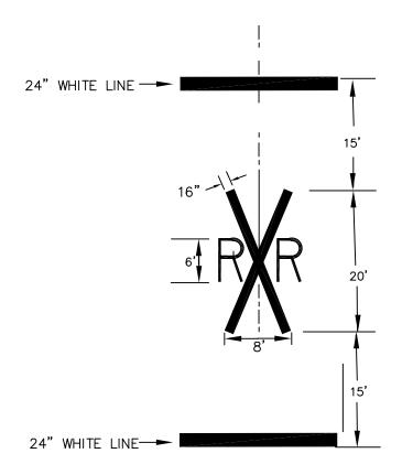
RAILROAD MARKINGS AT GRADE CROSSING: PAVEMENT MARKINGS IN ADVANCE OF A RAILROAD AT GRADE CROSSING SHALL CONSIST OF AN "X", THE LETTERS "RR", STOP BARS AND NO PASSING ZONE (DOUBLE YELLOW CENTER LINE OR RAISED MEDIAN). IDENTICAL MARKING SHALL BE PLACED IN EACH APPROACH LANE TO THE GRADE CROSSING.
