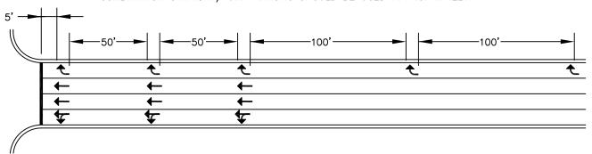
MERGE LANE ARROWS: STRAIGHT WHITE ARROWS AT 45° ANGLE TO THE LANE LINE SHALL BE INSTALLED IN THE THROUGH LANE THAT IS MERGED INTO AN ADJACENT THROUGH LANE AS SHOWN BELOW:
