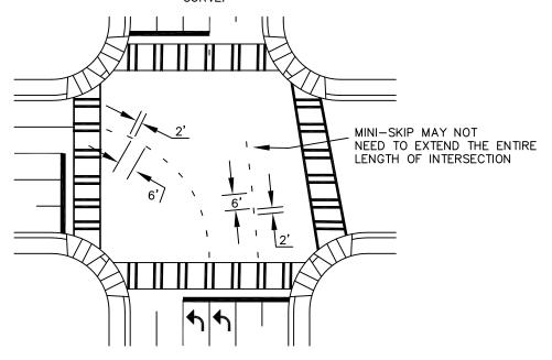
CENTER LINES SHALL BE A DOUBLE YELLOW LINE. A DOUBLE YELLOW LINE SHALL CONSIST OF TWO SOLID 4" SIDE YELLOW LINES PLACED 4" APART. WHEN WARRANTED, CENTER LINES SHALL BE USED TO SEPARATE TRAFFIC TRAVELING IN OPPOSITE DIRECTIONS WHERE A MEDIAN ISLAND IS NOT PRESENT. CENTER LINE MARKINGS SHALL BE PLACED ON STREETS THAT HAVE AN ADT OF 6000 VEHICLES PER DAY OR MORE AND ALSO ARE 20' OR MORE IN WIDTH.
