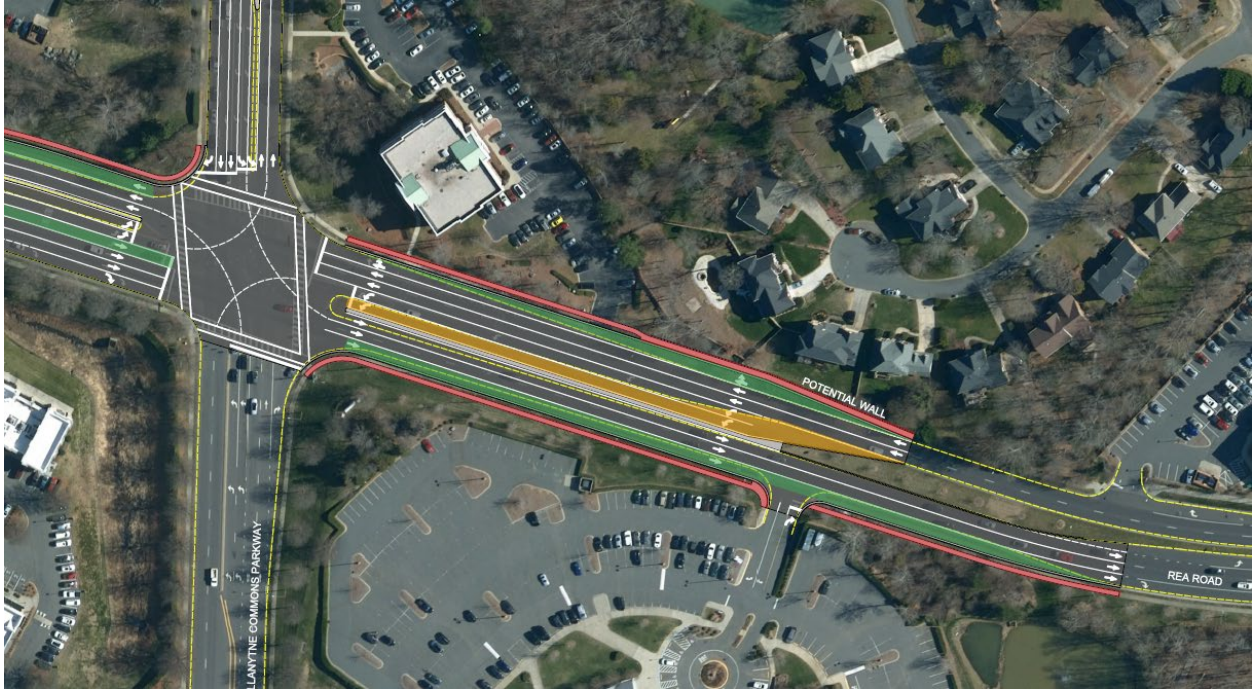
Rea Road and Ballantyne Commons Parkway Intersection (Green = new through lane; Orange = new or lengthened turn lane, Red = 6' wide sidewalk)
