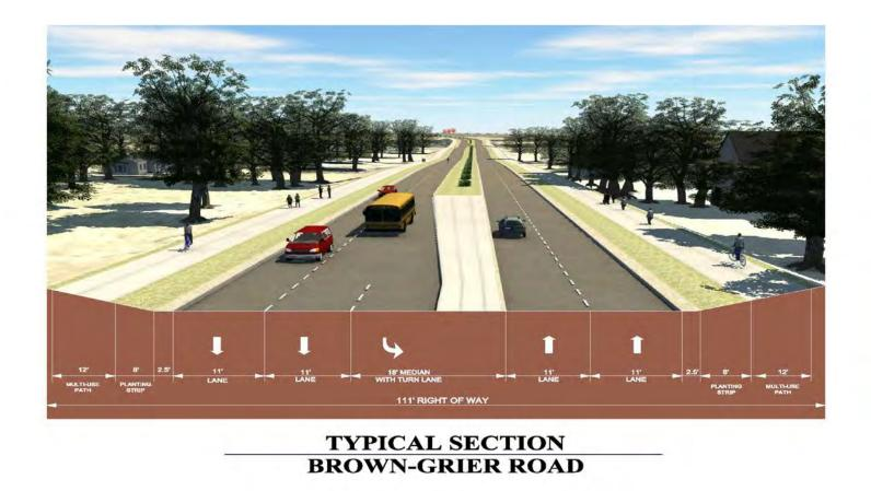
The Brown-Grier Road Upgrade will widen existing Brown Grier between the Arrowwood Road intersection to the Steele Creek Road intersection to a 4 lane median divides roadway with planting strips and multi-use paths along both sides.
