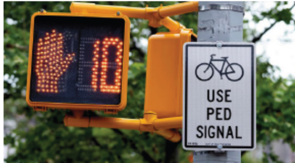
(Above) Leading pedestrian interval (LPI) installed in New York City, NY. Bicyclists use LPI to cross with pedestrians.
