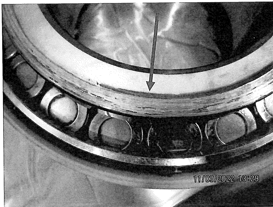
Figure 14 – Lubrication was also an issue for the intact tapered bearing. Note the blued metal (arrow) indicative of localized heating.
