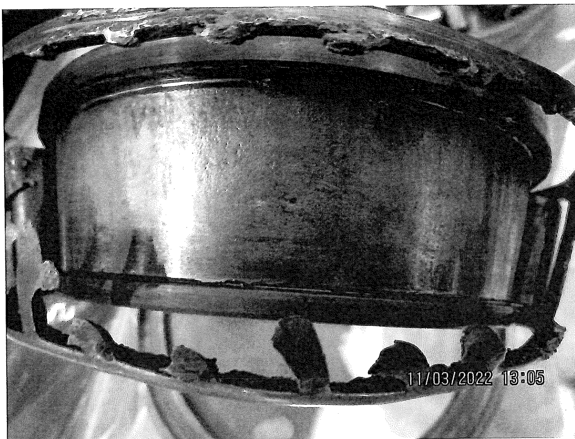
Figure 12 – the cylindrical roller after cleaning. The metal cage failed ends are all swept in the same direction. The missing pieces account for most of the debris found.
