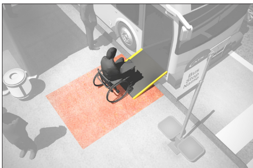
Boarding & Alighting Area
