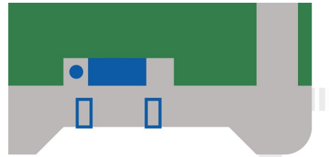
Figure 12. Depicts a scenario in which a pull-in was possible by cutting into the space normally dedicated to a planting strip and setback. An off-sidewalk space was paved on the adjacent property to accommodate placement of amenities.
