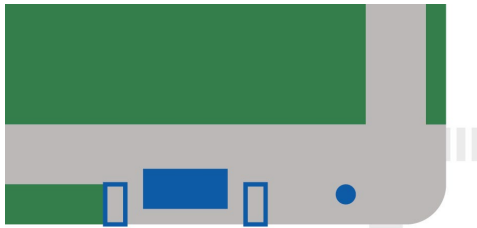
Figure 11. Depicts a scenario in which a bus stop had to remain “flush” with the roadway edge with no option for either a bulbout or pull-in. The planting strip was paved from the boarding area back to the crosswalk to accommodate placement of amenities.
