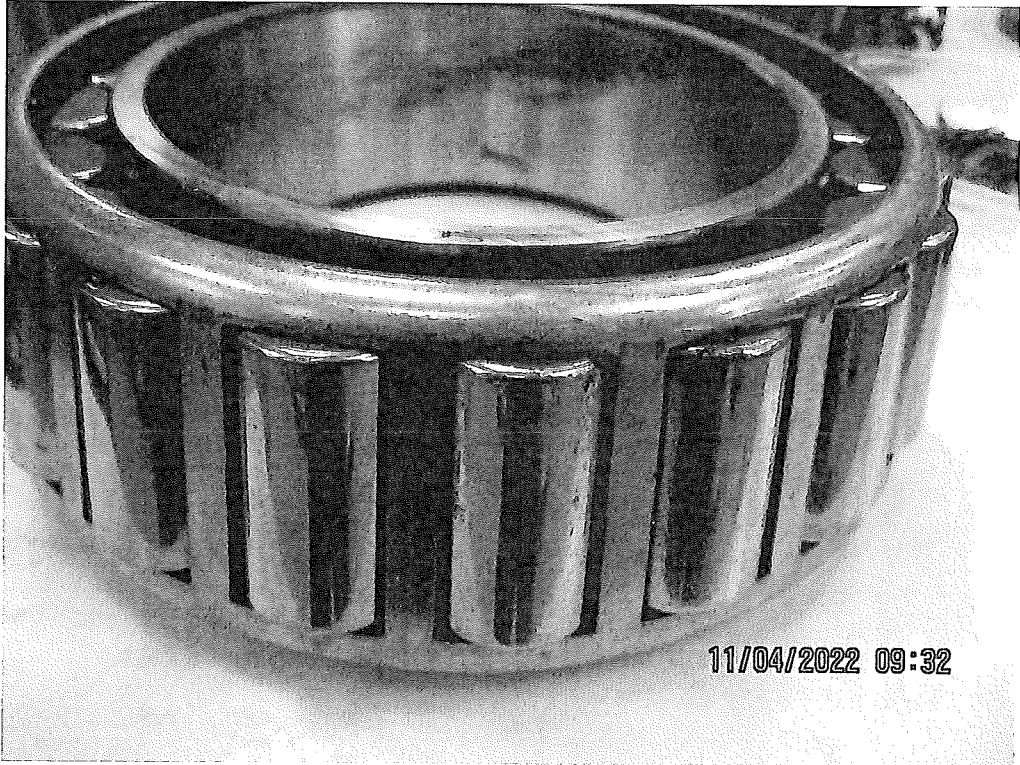
Figure 17 – even the intact tapered bearing displayed some localized corrosion.
