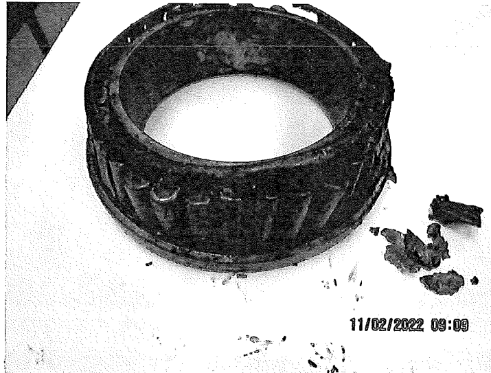
Figure 1: Disassembled smaller taper roller. This was the section with the greatest degree of damage. Much of the metal cage has been destroyed.
