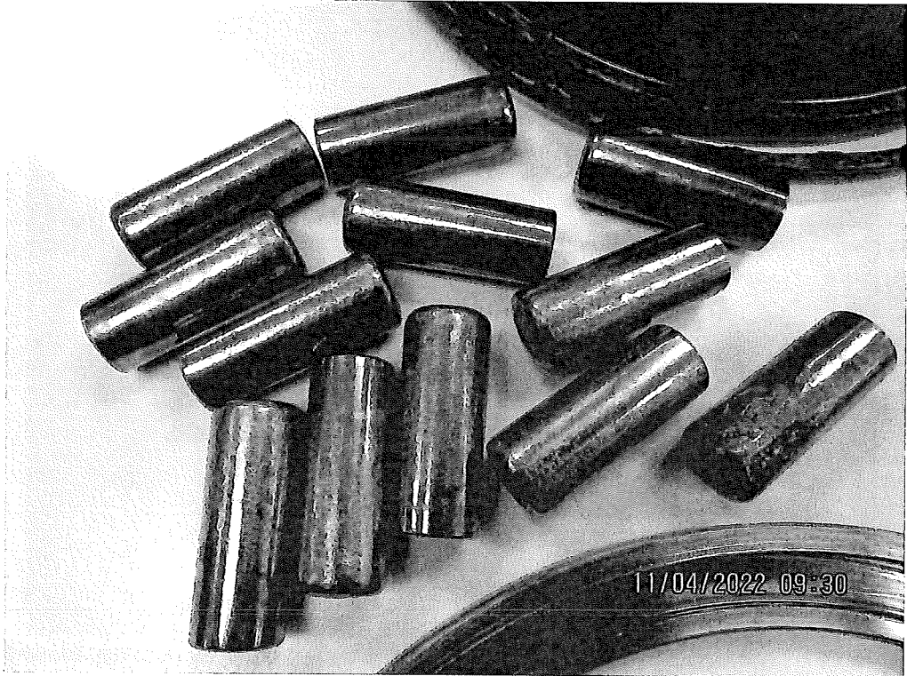
Figure 16 – a collection of cylindrical rollers after cleaning. Scoring, corrosion and bluing from heat is evident.
