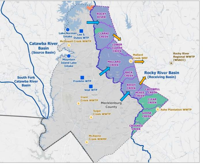
An IBT is a withdrawal, diversion or pumping of water from one source river basin to another river basin. The water from the source basin is treated and distributed to customers for everyday water usage, then collected and treated at wastewater treatment plants before portions are discharged to the receiving basin, resulting in the interbasin transfer.
