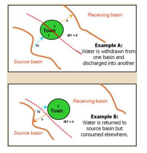
The amount of a transfer is determined by the amount of water moved from the source basin to the receiving basin, less the amount of water returned to the source basin and consumptive use in the source basin.
